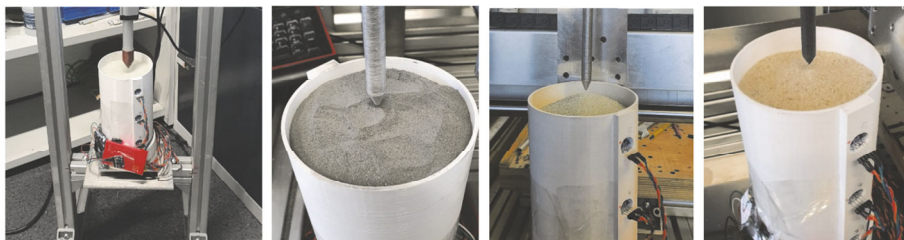
Figure 22: Preliminary setup (a) and tested materials: DNA-1A (b), glass beads (c), Ottawa sand (d).
