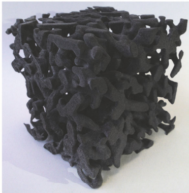
Figure 25: Upscaled and 3d-printed snow microstructure with an original edge length of 2 mm.
